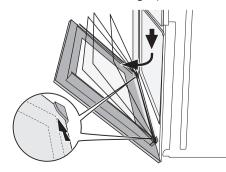
2. Hold the door strip (B) on both sides, align it with the inner edge of the door and press the door strip (B) into the upper edge of the door.
